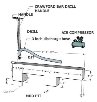
Consideration should be made to the location of the air compressor as it relates to the anticipated depth of the borehole and the length of the air hose. If the borehole is to be about 75 ft. deep and the hose is 100 ft then the compressor should be within 15 ft. of the borehole so that there is plenty of hose to spare when laying the Crawford Bar on the ground away from the mud pit. If the depth of the borehole is unknown, then spare hose should be on hand in case it is needed.
