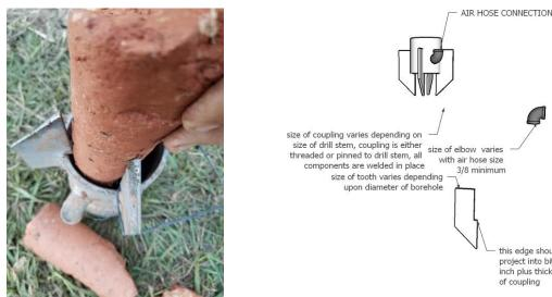
In the drawing on the right, the bit is built directly on a coupling and the air inlet is welded directly to the coupling. The teeth of the bit protrude a little over a <sup>1</sup>/<sub>4</sub> inch into the inlet of the portion of the bit that attaches to the drill stem. In most instances the bit can protrude even more, however, the more it protrudes the less room there is should the bit need to pass gravel or broken laterite.
