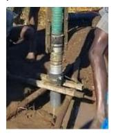
available in every country where I have worked. Sometimes it must be imported from a major city within a country. If one is drilling with a certain diameter drill stem, then the discharge hose should be the same interior diameter as the drill stem. The ideal situation is to connect the discharge hose with a connector that is the same size as
